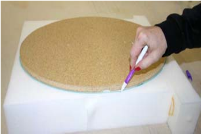
Using 4" thick foam, trace the oval shape of the base of stool onto the foam and cut. Cut-to-order foam is available from Textile Warehouse (1-800-281-9391).
