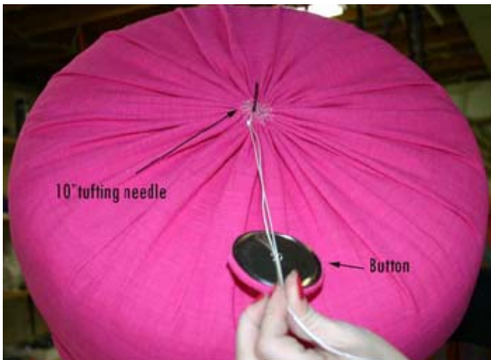
Cover a 2" diameter button with your fabric. Using a 10" tufting needle and tufting twine, thread the twine through the eye of the button and insert the threaded needle through the center of the cushion.
