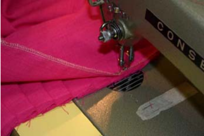
Sew the pleating to the right side of the skirt using a 1/2" seam allowance.
