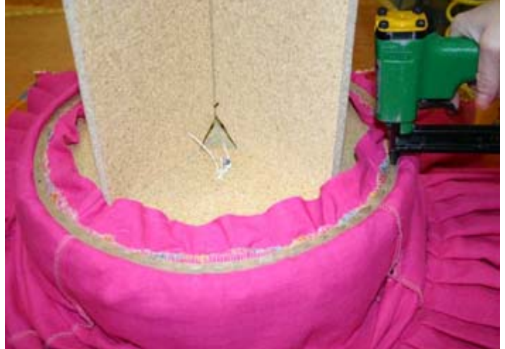
Staple the cardboard tacking strip next, lining up the outer edge with the edge of the particle board.. This gives you a rigid edge. Cardboard tacking strip is available at upholstery shops and at Textile Warehouse (1-800-281-9391)
