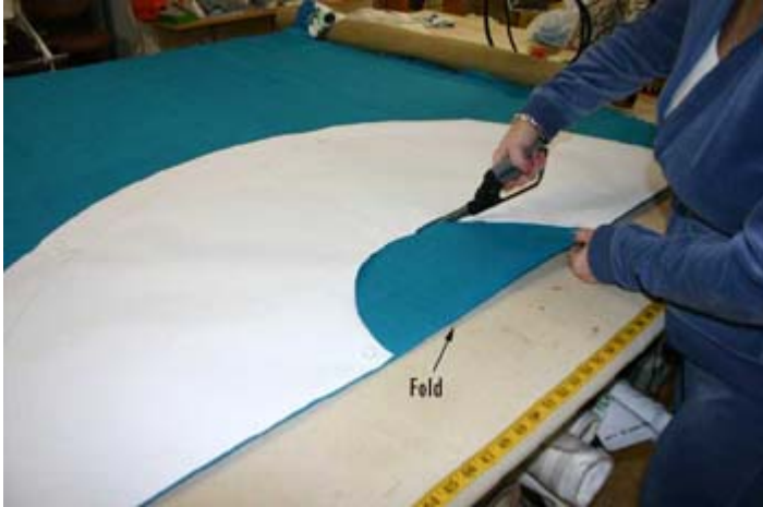
Placing the skirt pattern on the fold, cut out the bottom skirt layer
