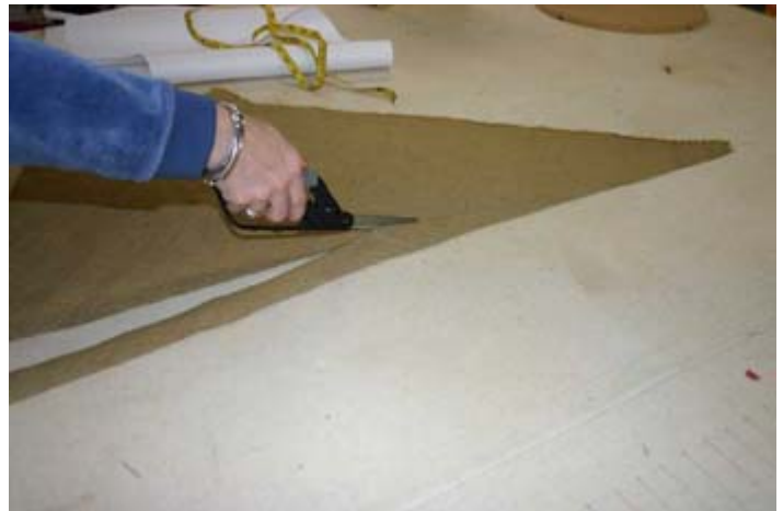
Cut the fabric to cover the piping on the bias. We use 4/32" piping and cut our pieces about 1-3/4" wide. Cut enough to go around the bottom of the skirts.
