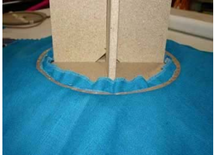
Staple cardboard tacking strip next, lining up the outer edge with the edge of the particle board. This gives you a rigid edge. Cardboard tacking strip is available at upholstery supply shops and at Textile Warehouse (770-381-1199).
