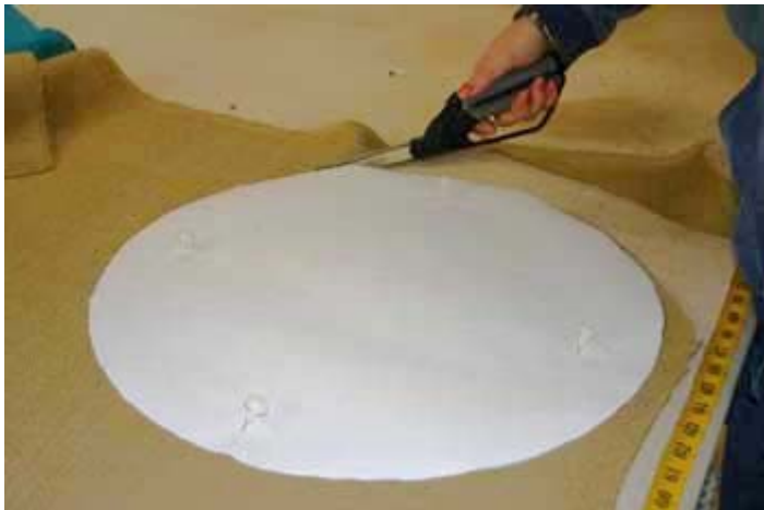
Pin the cushion top pattern onto fabric and cut. The seam allowances have been added to the pattern.
